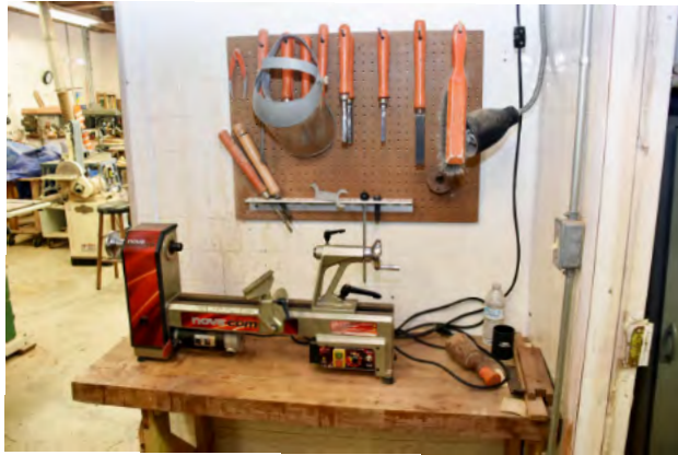
One of the wood lathes used to make pens out of exotic woods.
