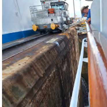
Photos submitted by Carole Young The "Mule" seen on the left helps keep ships centered while traversing the canal.
