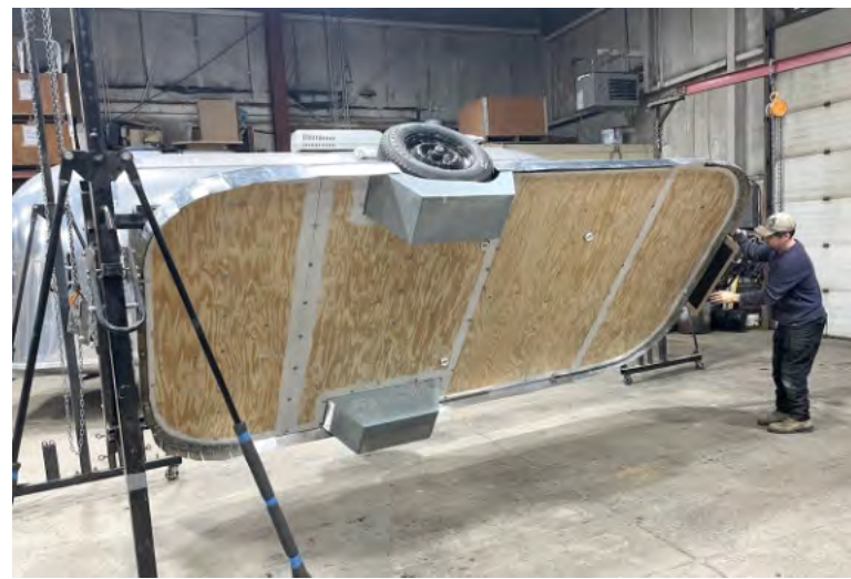
Colin's "rotisserie" setup to allow for a full shell-off restoration in which he spins the chassis to work on it.
